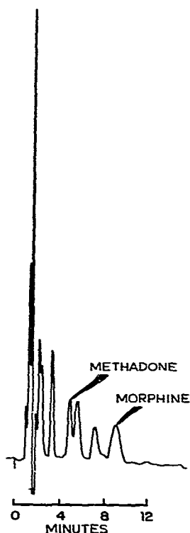
Fig. 5. Determination of morphine and methadone in urine. See Table V for the measured ratios. Conditions: column, fluoro ether SIL-X-I, 2.6 mm \times 50 cm; eluent, water-acetonitrile containing 0.3% \text{H}_3\text{PO}_4 (8:92); flow-rate, 2 ml/min; inlet pressure, 600 p.s.i.g.; temperature, 70°; detection, 210 nm (0.1 a.u.f.s.).
